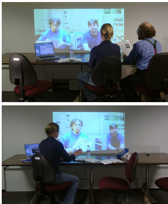
Figure 6: View dependent effect when the local conferees move to different spots. Smaller images show the synthesized views. Notice that we have placed a book in the scene. When the local conferees are at right, as in the top image, the view point of the synthesized view is from the right, revealing the front cover of the book. When the conferee moves to left, as in the bottom image, the view changes accordingly, revealing the back cover of the book.
